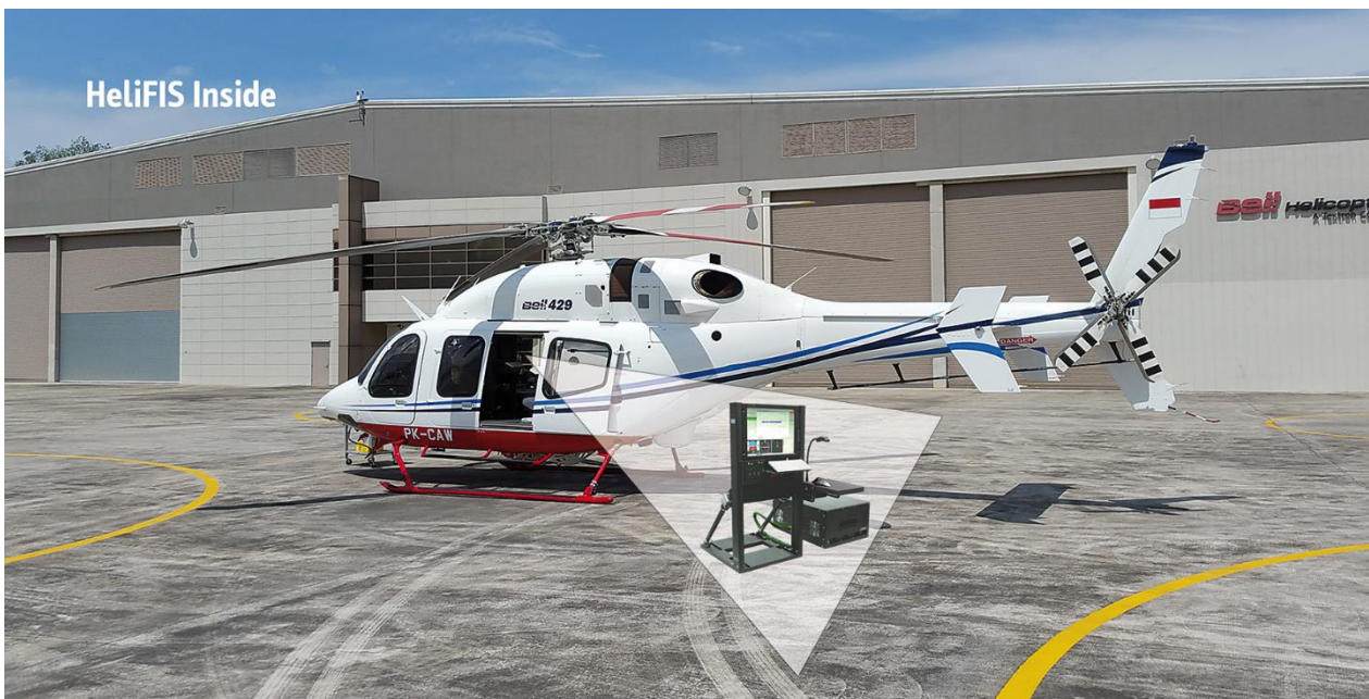
Bell 429 helicopter with Flight Inspection System HeliFIS®
