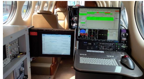
AD-AFIS-255 installed in KingAir 350i
