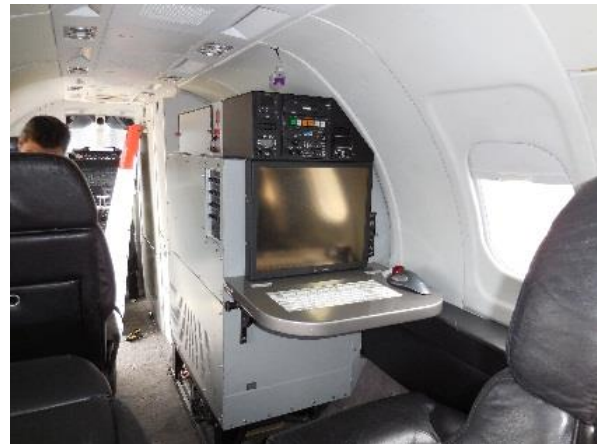
AeroFIS® installed in Argentinean LearJet 35A
