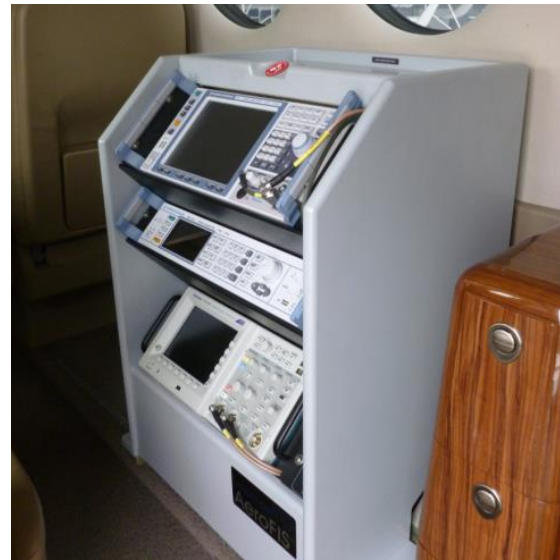
Equipment Console installed in King Air
