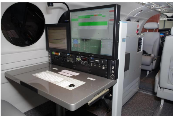
AeroFIS® installed in PANSa King Air 350
