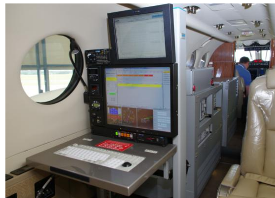
AeroFIS® Installed in CAA Taiwan KingAir B350iER
