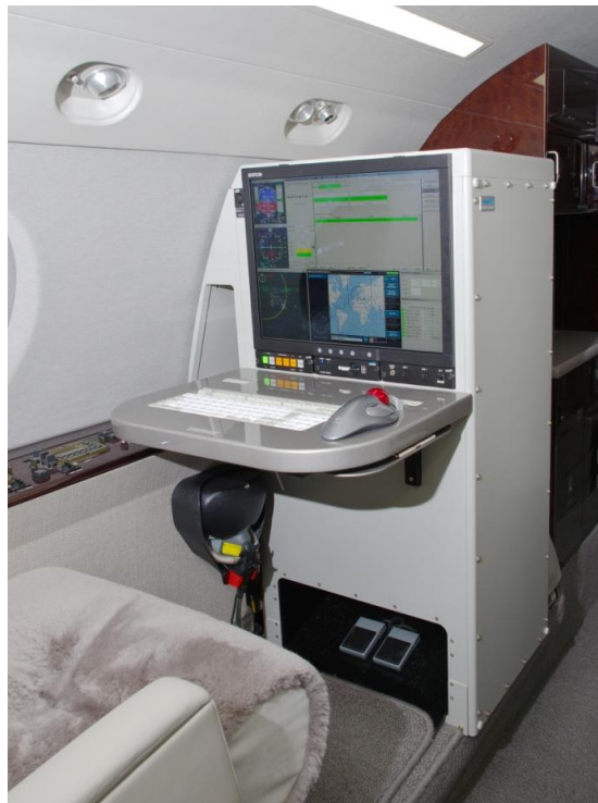
AeroFIS Installed in RNoAF Falcon 20
