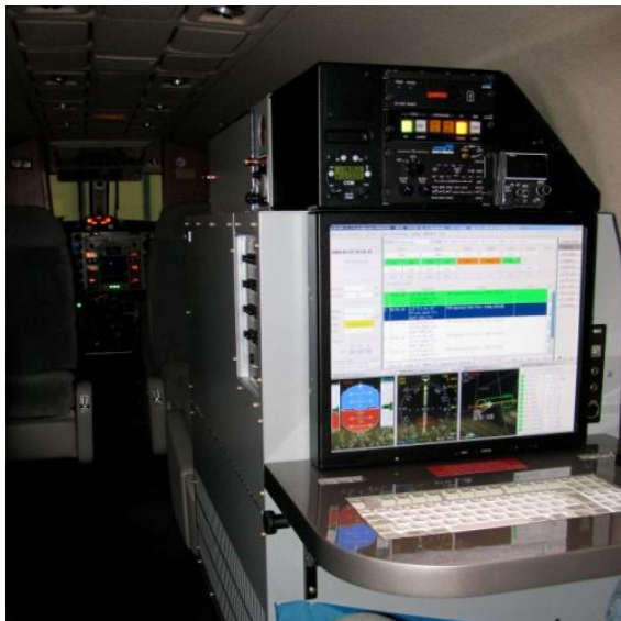
AeroFIS installed in KingAir 350i
