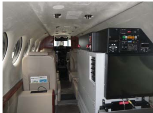
AeroFIS installed in a King Air 350i
