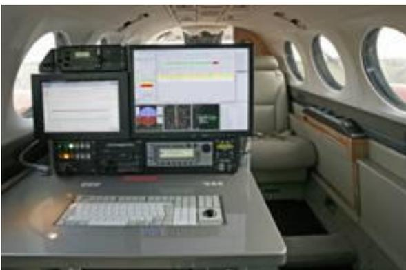
AeroFIS installed in new Super King Air 350
