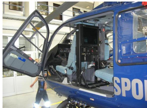
Workstation installed in EC135
