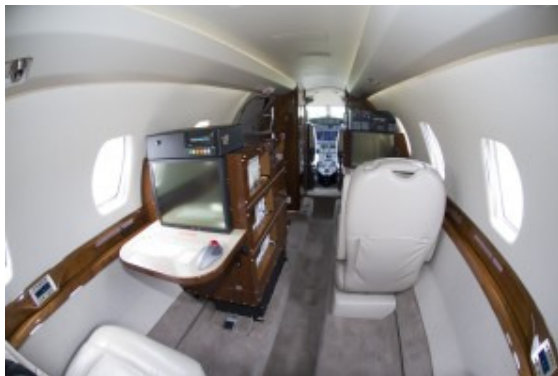
Aerodata FIS installed in Citation X
