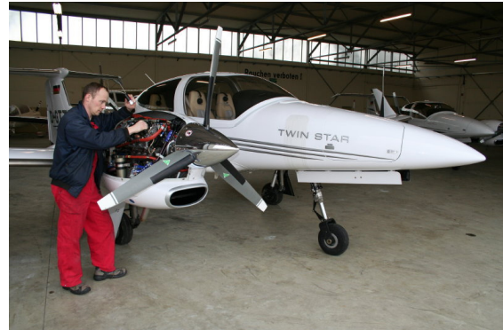
Engine Inspection on Diamond DA-42
