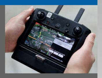
The planed flight inspection procedures are directly transmitted into the drone pilot's AeroFIS® Flybot Remote Control software. It provides a map view of the drone position and the flight procedure, and a first person camera view of the drone to the pilot.
